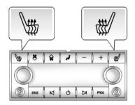
With the ignition in ON/RUN/START, press of to heat the left or right seat cushion and seatback. An indicator on the RSA display appears when this feature is on.
